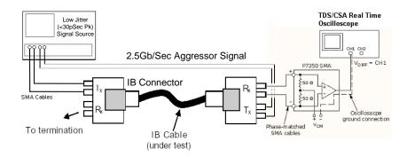
Figure 16 – Test Setup for IB cable testing.
