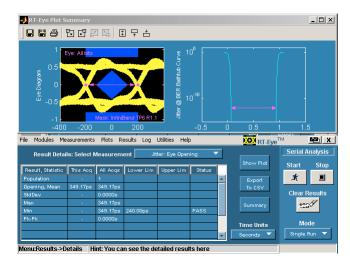
Figure 13 - Results of the Jitter Eye Opening @ 10<sup>-12</sup> BER Measurement.
