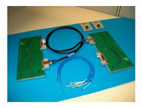
Figure 15 – Gore cable test fixture.
