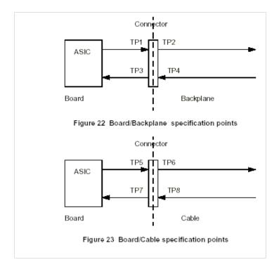
Figure 1 – Compliance Points from InfiniBand Specification.
