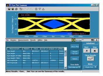
Figure 9 - Result of the Differential Amplitude Measurement.
