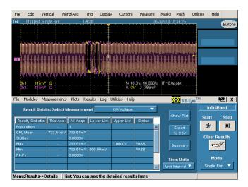
Figure 7 - Result of the DC Common Mode Measurement.
